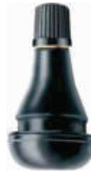
**VÁLVULA PARA PNEUS SEM CÂMARA**
